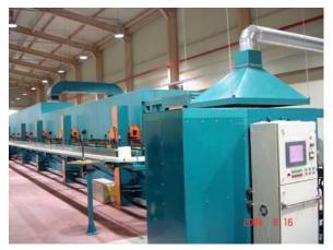
High pressure P.U. foam dispensing machine complete with: VOLTAGE: THREE PHASE, 380V, 50HZ
