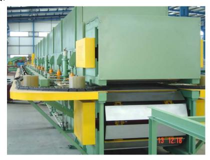
• One set of heating and heat insulation system: the DOUBLE BELT machine is closed by heat insulation material. The heating system heat and fan hot air to keep the temperature 25-35°C in the DOUBLE BELT machine. The temperature could adjust according to the production process.
