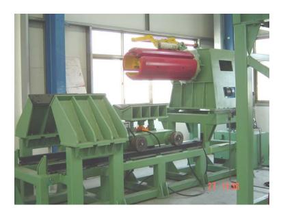
Two sets of steel sheet transverse cutting machine: it is hydraulic, could cut steel sheet according to certain length and move by the sheet running.两套钢板横切断装置,在开卷装置后面,采用液压驱动切断钢板的方式,可实现计长和定长切断,可随钢板同步运动:
